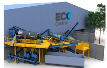
Figure 1: EcoCentral Glass Pulverising Plant
