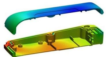
Figure 2: Casing Seal and Displacement Analysis
